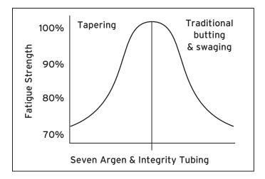
In addition, the properties of an internally butted titanium tube are affected by the excessive manipulation that occurs when using a mandrel. Although cold working can increase strength, too much cold working after the tube mill's final annealing and stress relieving cycles can detrimentally change the texture of the tubing. The tubing's CSR (Contractile Strain Ratio) increases-beyond its optimal rate-resulting in poor fatigue characteristics.
