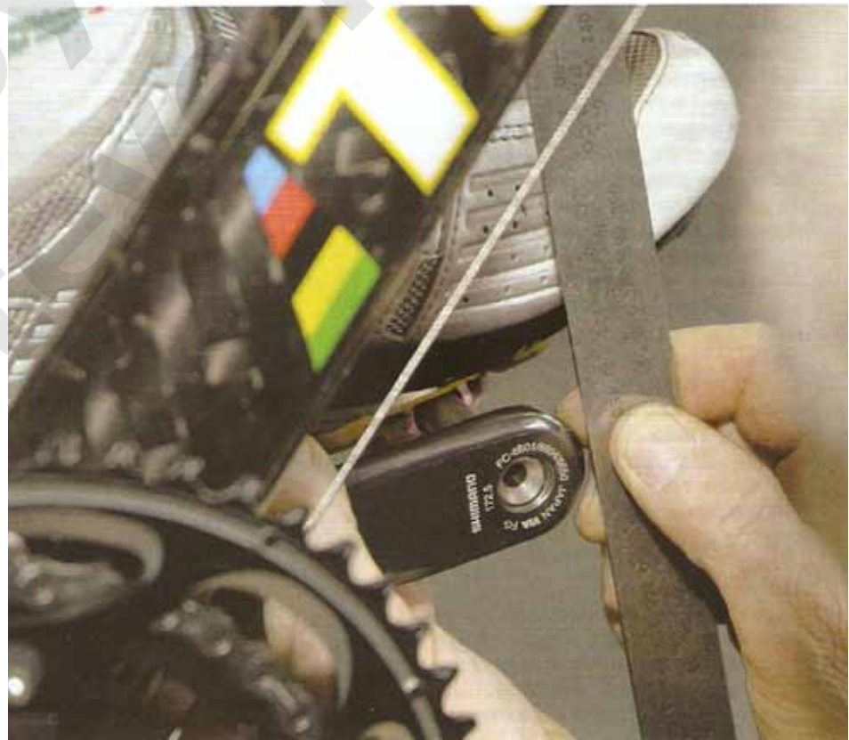
Installation of wedges takes a lot of time. Both the inside and outside foot have to be measured and the correct angle decided upon.
